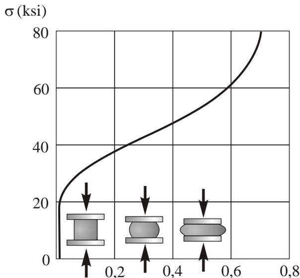
Fig. 22 Stress-strain diagram for copper in compression
