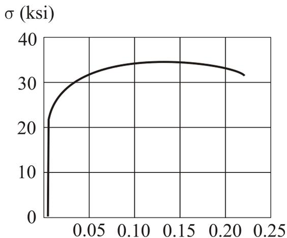
Fig. 19 Typical stress-strain diagram for an aluminum alloy
