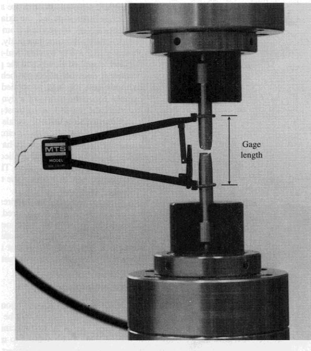
Fig. 6 Typical tensile-test specimen with extensometer attached. The specimen has just fractured in tension.
