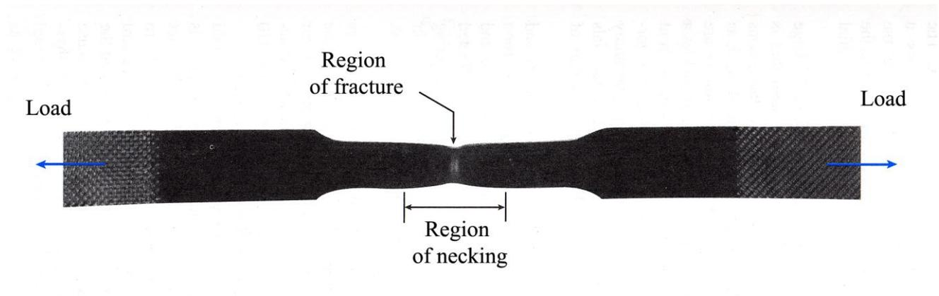
Fig. 17 Necking of a mild-steel bar in tension
