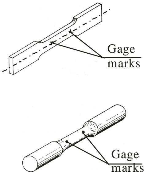
Fig. 3 Types of test specimens
