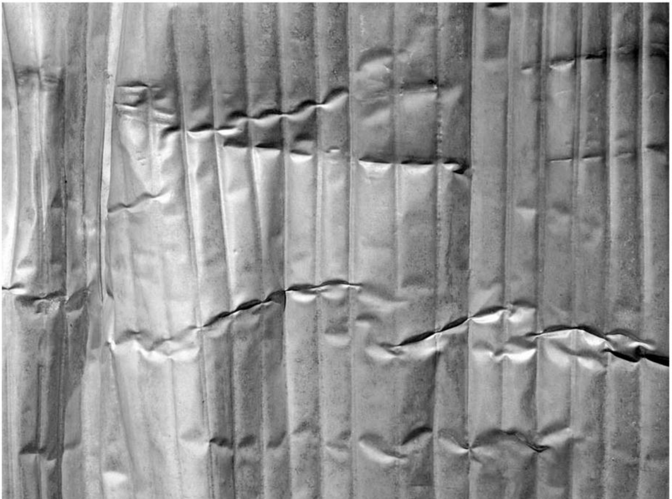
Fig. 3 (a) Unbuckled and (b) buckled configuration of compressed posts; (c) image of buckled compressed skin
