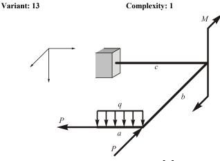
Given: q = 10 kN/m; P = 20 kN; M = 10 kNm;  $[\sigma] = 160 \text{ MPa}$ ; a = 2 m,  $b = 3 \,\mathrm{m}; \ c = 4 \,\mathrm{m}.$
