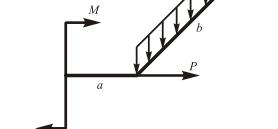
Given: q = 10 kN/m; P = 20 kN; M = 10 kNm;  $[\sigma] = 160 \text{ MPa}$ ; a = 2 m, b = 3 m; c = 4 m.
