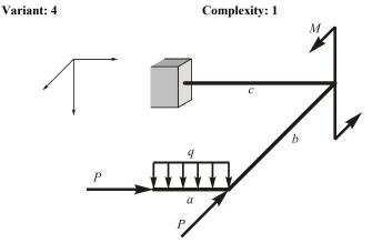
Given: q = 10 kN/m; P = 20 kN; M = 10 kNm;  $[\sigma] = 160 \text{ MPa}$ ; a = 2 m, b = 3 m; c = 4 m.
