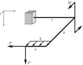
Given: q = 10 kN/m; P = 20 kN; M = 10 kNm;  $[\sigma] = 160 \text{ MPa}$ ; a = 2 m, b = 3 m; c = 4 m.
