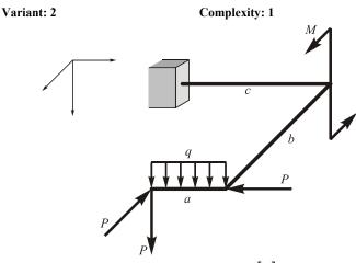
Given: q = 10 kN/m; P = 20 kN; M = 10 kNm;  $[\sigma] = 160 \text{ MPa}$ ; a = 2 m, b = 3 m; c = 4 m.
