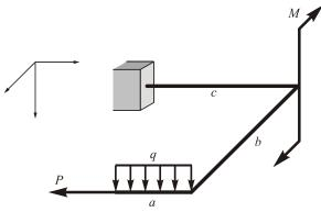
Given: q = 10 kN/m; P = 20 kN; M = 10 kNm;  $[\sigma] = 160 \text{ MPa}$ ; a = 2 m,  $b = 3 \,\mathrm{m}; \ c = 4 \,\mathrm{m}.$
