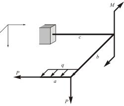
Given: q = 10 kN/m; P = 20 kN; M = 10 kNm;  $[\sigma] = 160 \text{ MPa}$ ; a = 2 m, b = 3 m; c = 4 m.
