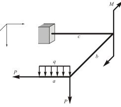
Given: q = 10 kN/m; P = 20 kN; M = 10 kNm;  $[\sigma] = 160 \text{ MPa}$ ; a = 2 m, b = 3 m; c = 4 m.
