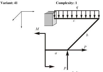
Given: q = 10 kN/m; P = 20 kN; M = 10 kNm;  $[\sigma] = 160 \text{ MPa}$ ; a = 2 m,  $b = 3 \,\mathrm{m}; \ c = 4 \,\mathrm{m}.$
