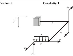
Given: q = 10 kN/m; P = 20 kN; M = 10 kNm;  $[\sigma] = 160 \text{ MPa}$ ; a = 2 m,  $b = 3 \,\mathrm{m}; \ c = 4 \,\mathrm{m}.$
