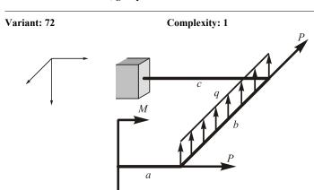
Given: q = 10 kN/m; P = 20 kN; M = 10 kNm;  $[\sigma] = 160 \text{ MPa}$ ; a = 2 m, b = 3 m; c = 4 m.
