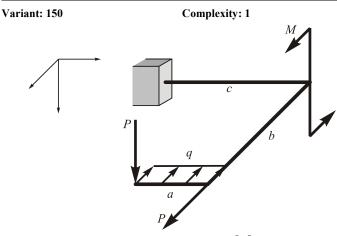
Given: q = 10 kN/m; P = 20 kN; M = 10 kNm;  $[\sigma] = 160 \text{ MPa}$ ; a = 2 m,
