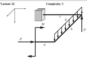
Given: q = 10 kN/m; P = 20 kN; M = 10 kNm;  $[\sigma] = 160 \text{ MPa}$ ; a = 2 m, b = 3 m; c = 4 m.
