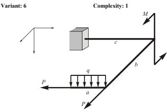
Given: q = 10 kN/m; P = 20 kN; M = 10 kNm;  $[\sigma] = 160 \text{ MPa}$ ; a = 2 m,
