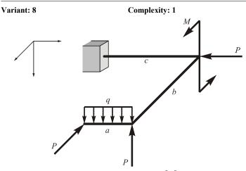
Given: q = 10 kN/m; P = 20 kN; M = 10 kNm;  $[\sigma] = 160 \text{ MPa}$ ; a = 2 m, b = 3 m; c = 4 m.
