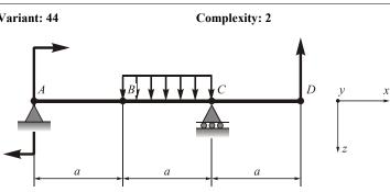
Given: q = 10 kN/m; P = 20 kN; M = 10 kNm;  $E = 2 \times 10^{11} \text{ Pa}$ ;  $[\sigma] = 160 \text{ MPa}; a = 2 \text{ m}.$
