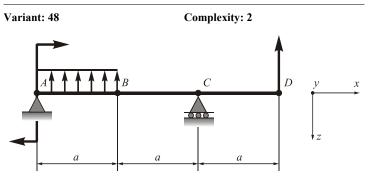
Given: q = 10 kN/m; P = 20 kN; M = 10 kNm;  $E = 2 \times 10^{11} \text{ Pa}$ ;  $[\sigma] = 160 \text{ MPa}$ ; a = 2 m.
