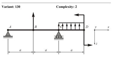
Given: q = 10 kN/m; P = 20 kN; M = 10 kNm;  $E = 2 \times 10^{11} \text{ Pa}$ ;  $[\sigma] = 160 \text{ MPa}$ ; a = 2 m. Goal:
