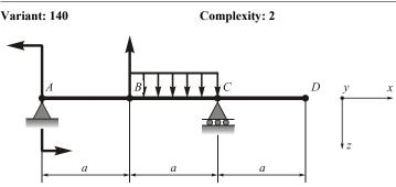
Given: q = 10 kN/m; P = 20 kN; M = 10 kNm;  $E = 2 \times 10^{11} \text{ Pa}$ ;  $[\sigma] = 160 \text{ MPa}; a = 2 \text{ m}.$
