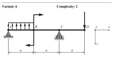
Given: q = 10 kN/m; P = 20 kN; M = 10 kNm;  $E = 2 \times 10^{11} \text{ Pa}$ ;  $[\sigma] = 160 \text{ MPa}$ ; a = 2 m. Goal:
