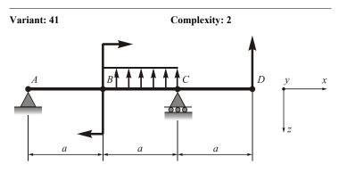
Given: q = 10 kN/m; P = 20 kN; M = 10 kNm;  $E = 2 \times 10^{11} \text{ Pa}$ ;
