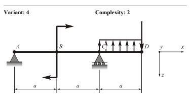
Given: q = 10 kN/m; P = 20 kN; M = 10 kNm;  $E = 2 \times 10^{11} \text{ Pa}$ ;  $[\sigma] = 160 \text{ MPa}$ ; a = 2 m.
