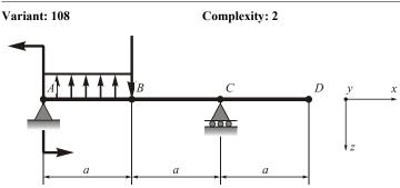
Given: q = 10 kN/m; P = 20 kN; M = 10 kNm;  $E = 2 \times 10^{11} \text{ Pa}$ ;  $[\sigma] = 160 \text{ MPa}$ ; a = 2 m.
