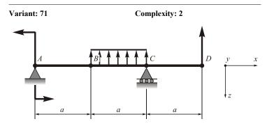
Given: q = 10 kN/m; P = 20 kN; M = 10 kNm;  $E = 2 \times 10^{11} \text{ Pa}$ ;
