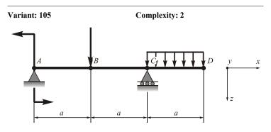
Given: q = 10 kN/m; P = 20 kN; M = 10 kNm;  $E = 2 \times 10^{11} \text{ Pa}$ ;
