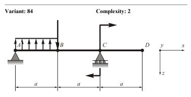
Given: q = 10 kN/m; P = 20 kN; M = 10 kNm;  $E = 2 \times 10^{11} \text{ Pa}$ ;  $[\sigma] = 160 \text{ MPa}; a = 2 \text{ m}.$
