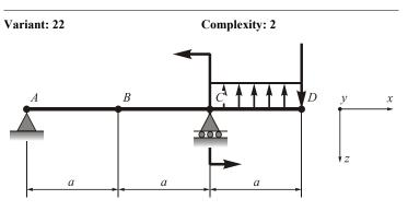
Given: q = 10 kN/m; P = 20 kN; M = 10 kNm;  $E = 2 \times 10^{11} \text{ Pa}$ ;  $[\sigma] = 160 \text{ MPa}; a = 2 \text{ m}.$ Goal:
