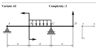
Given: q = 10 kN/m; P = 20 kN; M = 10 kNm;  $E = 2 \times 10^{11} \text{ Pa}$ ;  $[\sigma] = 160 \text{ MPa}; a = 2 \text{ m}.$ Goal:
